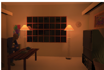
Proposed lighting scheme with high CS by day and low CS at night.
